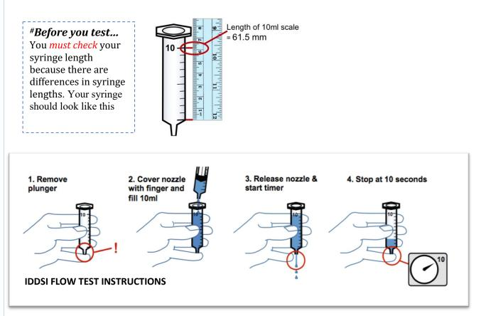
NOTE: Before use, check the nozzle is clear and free from any plastic residue or manufacturing defects that very occasionally occur.
